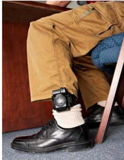
Figure 3. An ankle-worn alcohol detector (source: BI Incorporated)
